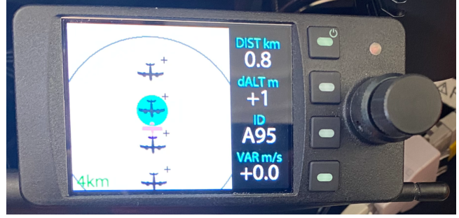
Figure 7: Four spoofed aircraft targets flying past the PowerFLARM Fusion receiver in a straight line.
