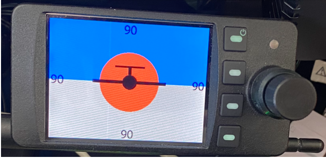
Figure 8: The PowerFLARM Fusion receiver strongly warns the pilot of a potential head-on collision.
