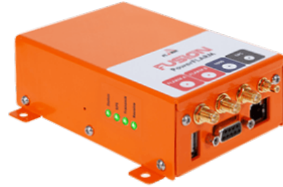
Figure 1: PowerFLARM Fusion. As one of the two main products of FLARM Technology, it can be installed on aircraft.
